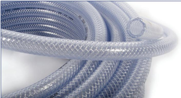
An economical, light duty hose ideal for multi-purpose use, PVK Glass Clear is especially popular for industrial airline equipment. It can also be used for food contact applications. Manufactured from transparent, low toxic PVC and reinforced with high tensile polyester fibres.
